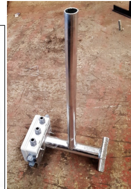
Junction box and warning light arm
